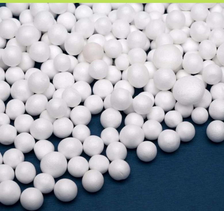
COMPOSÉ DE 98% D'AIR, LE POSYTE EST INERTE, BIOLOGIQUEMENT NEUTRE ET STABLE DANS LE TEMPS.
